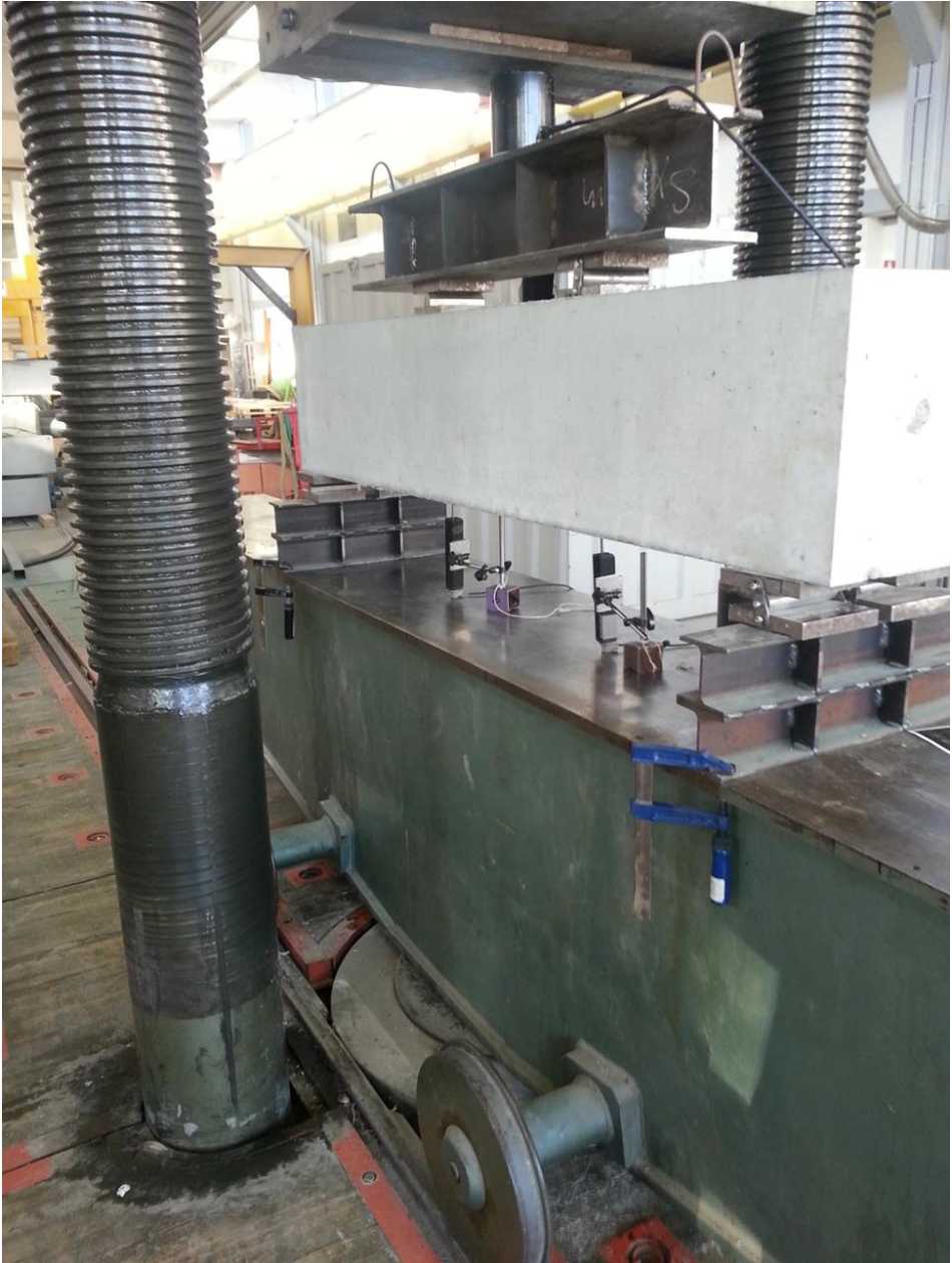
Figure 5. Four point bending tests, deformation controlled, on steel fiber reinforced concrete beams.
