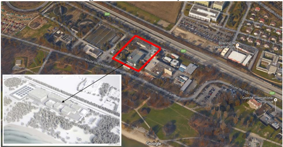
Figure 11: Architectural view model of the new sewage treatment plant in Lausanne and the model perimeter for simulating an excavation next to the incineration building.
