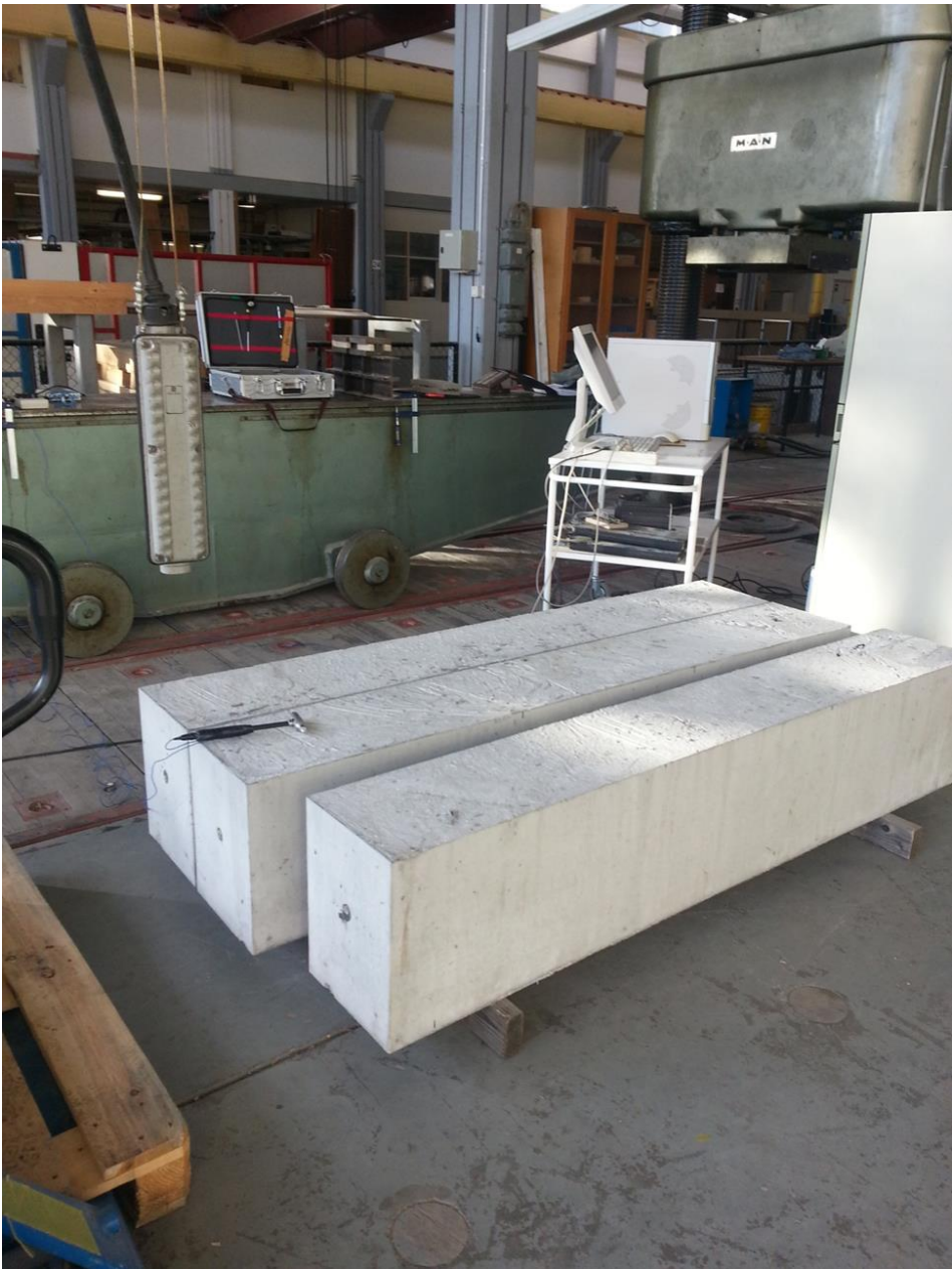
Figure 6. The resonance frequency is determined with seismic measurements.
